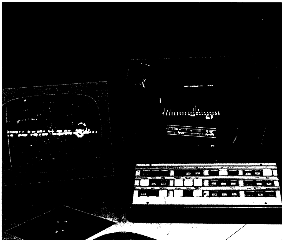
Display screens showing the Oxford PEPR in action sorting out two closely spaced tracks on film from the CERN 2 m bubble chamber. The screen on the left shows the two lines of bubbles recorded on the film. The screen on the right shows what PEPR has made of it. As a measure of the scale, the two 'peaks' marked above the two parallel lines of figures at the centre of the screen are about 100 \mu\text{m} apart. The limit of the resolution of the device is 25 to 30 \mu\text{m} which is close to the normal bubble diameter.
